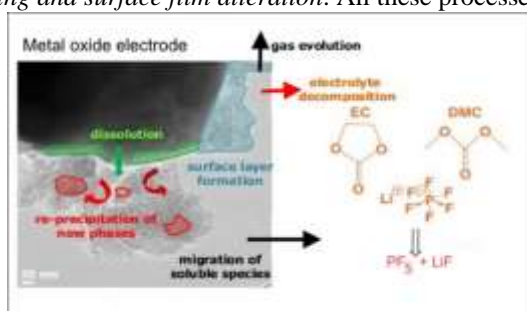
Figure 4. Schematic representation of ageing effect inside positive electrode [29].
